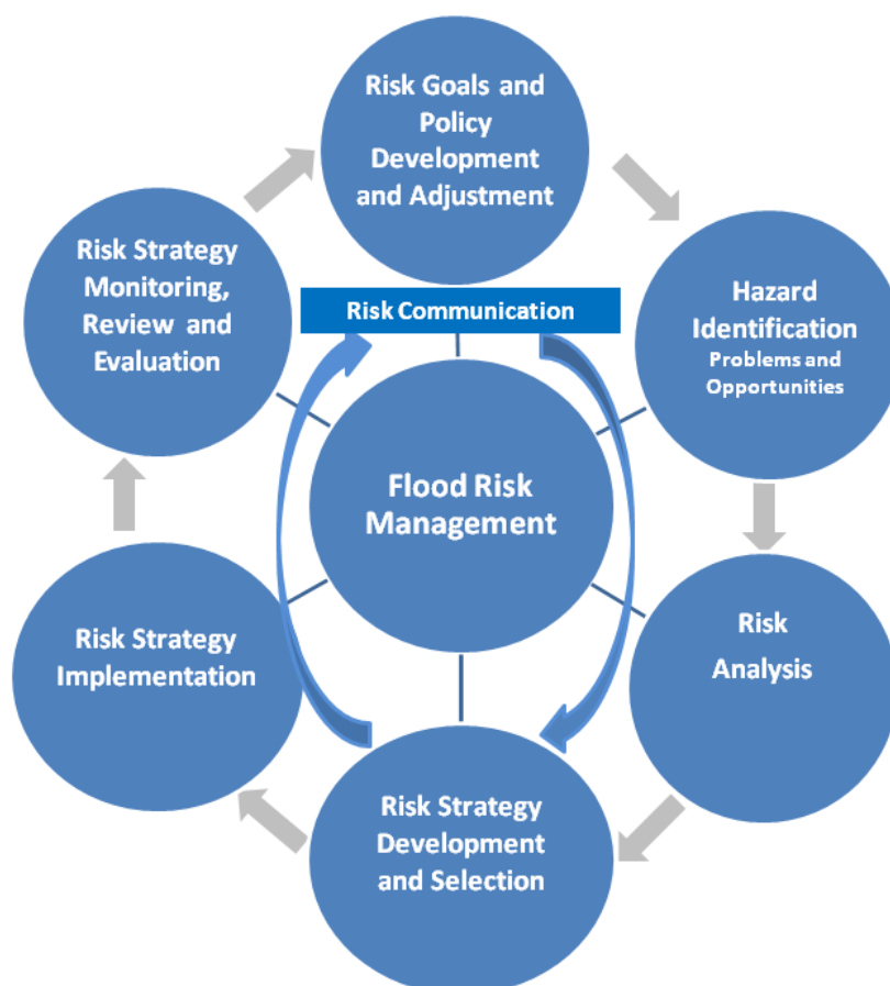
FIGURE 3-3: The flood risk management cycle illustrates the multi-step flood risk management process. SOURCE: Sayers et al., in press; NRC, 2012b; Moser et al., n.d.
