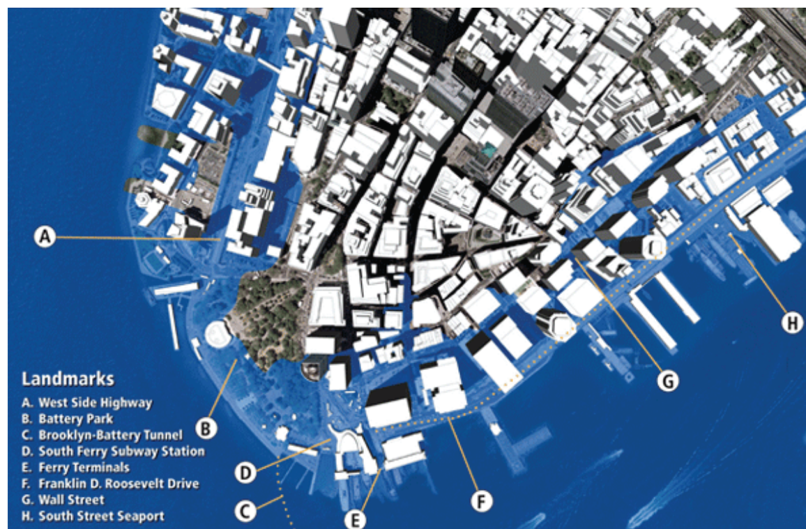
FIGURE 6-10: The challenge of rising sea level and the expansion of the one percent annual chance floodplain to New York City. The light blue area represents a 2012 depiction of the one percent annual chance floodplain of Lower Manhattan, New York City. With sea-level rise, a far larger area would be flooded in the event of a one percent annual chance flood event. (Note, flooding during Hurricane Sandy (2012) exceeded the one percent annual chance floodplain.) With sea-level rise, the one percent annual chance flood will inundate a larger area of New York City (not pictured here). SOURCE: USGCRP, 2009.
