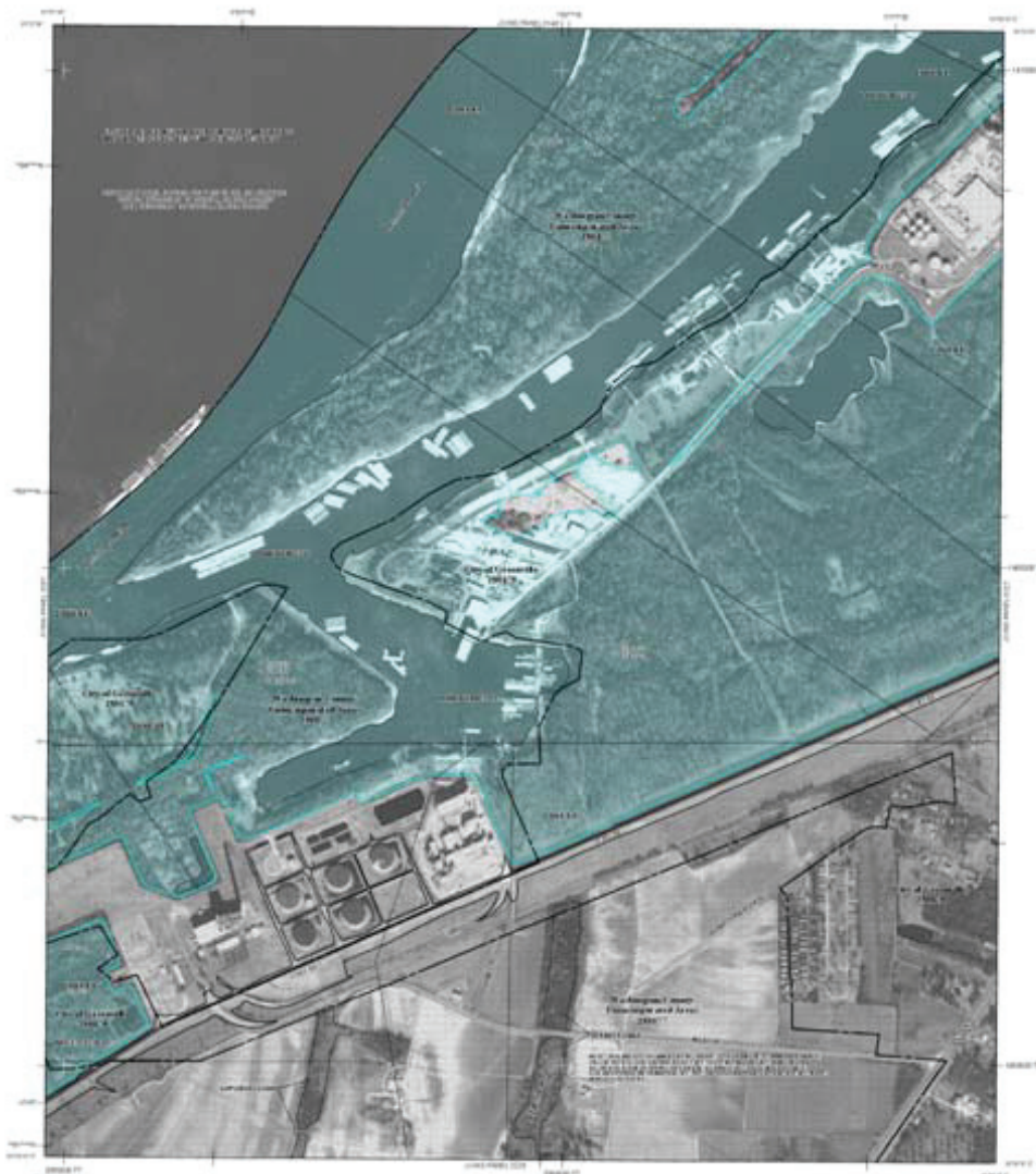
FIGURE 7-2: A Flood Insurance Rate Map for a section of Greenville, MS, along the Mississippi River. The blue areas are within the SFHA (Zone AE) and the gray area (Shaded Zone X) represents areas behind accredited levees.
